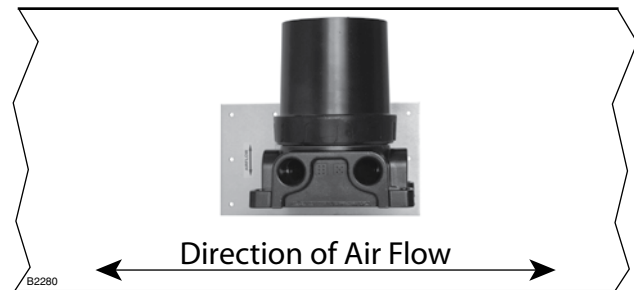
Figure 7—Orientation of PIRDUCT Mounting Plate Relative to Direction of Airflow through Duct
